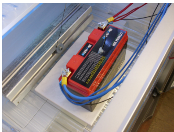
Figure 1: Deep-discharge cycle test in climate cabinet with the batteries 710003 (test at 0°C) and 710009 (test at 40°C)
