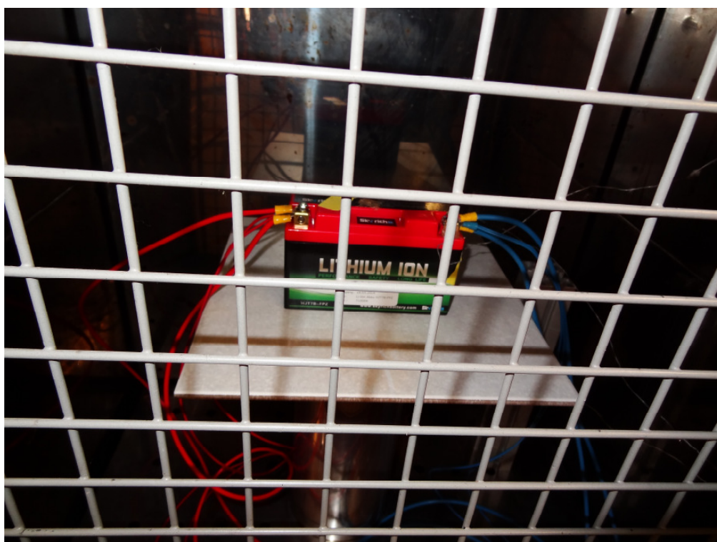
Figure 6: Short circuit test in climate cabinet with the batteries inside
