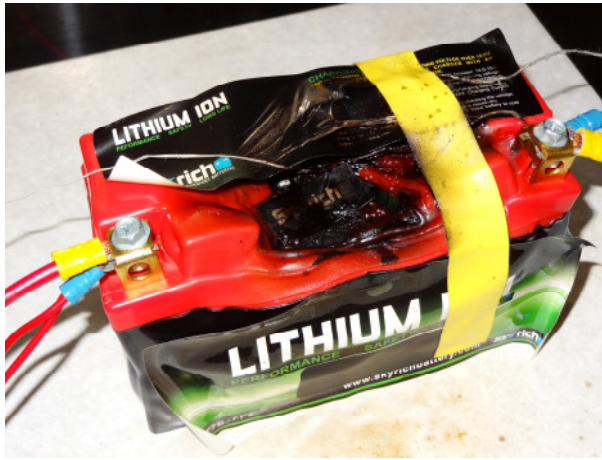
Figure 5: Overcharge test in safety cabinet with battery 710001 (overcharge current 30 A, overcharge voltage 100 V)
