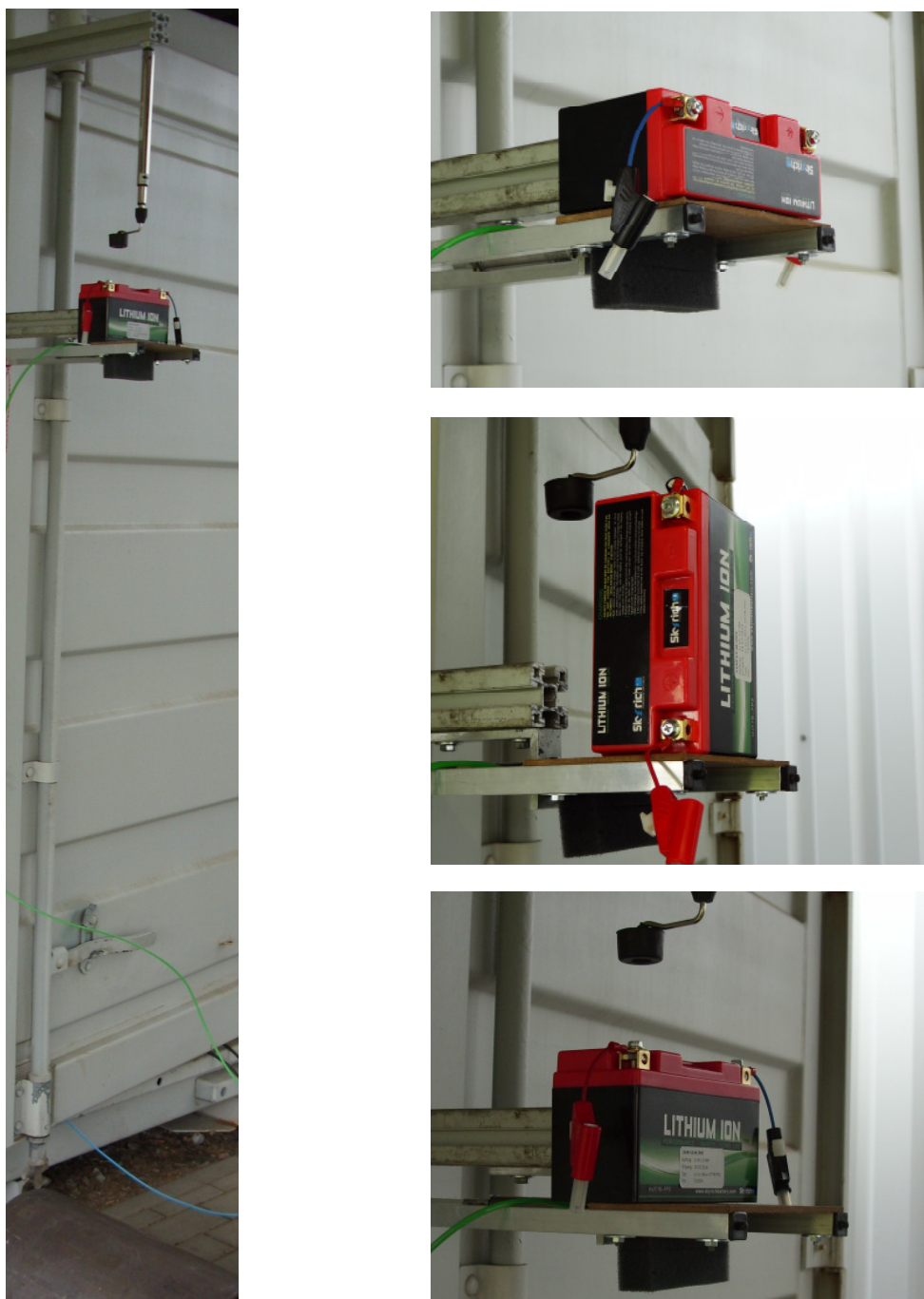
Figure 8: Pictures of the drop test
