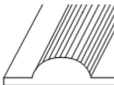
Abbildung 2: Waved surface of one of the crush plates.
