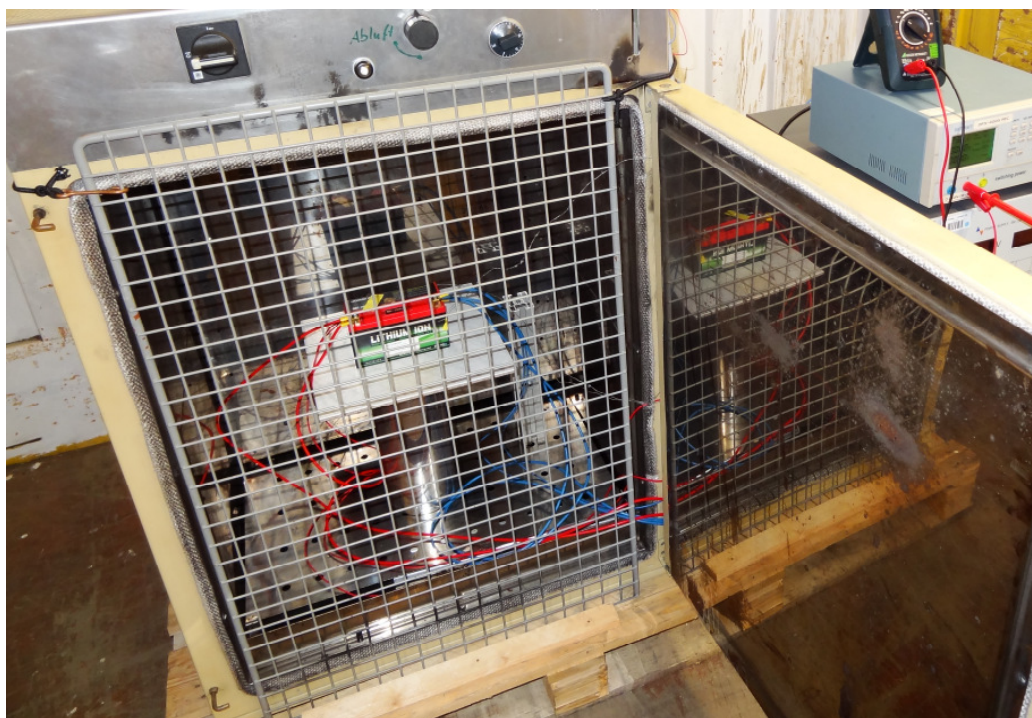
Figure 3: Overcharge test in climate cabinet with the batteries inside
