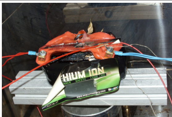
Figure 15: Heating test in climate cabinet with the battery 710008 inside (after the test with 140°C)
