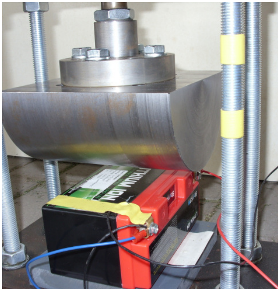
Figure 18: Battery at crush test apparatus
