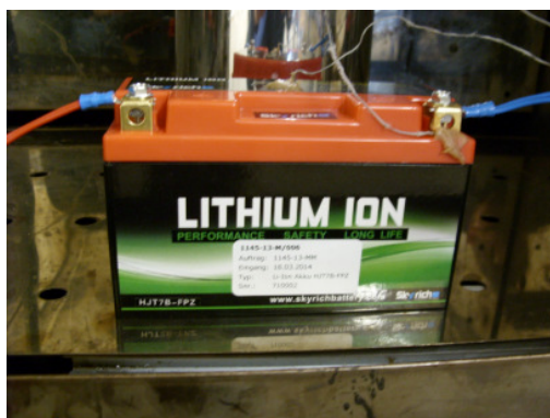
Figure 11: Heating test in climate cabinet with the batteries inside
